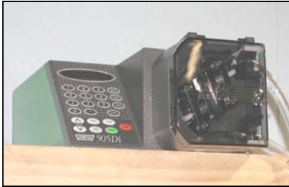
Computerized and metered delivery system for hydraulic fluid to all jacks insures the optimum operation of each jack when it leaves our factory.
