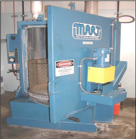
Our industrial parts washer is used to power wash every component that goes into our jacks to eliminate as much contamination to the internal workings of the jack as is possible to insure the longevity of our equipment in the field.
