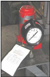
Master gages, re-calibrated and re-certified annually.
