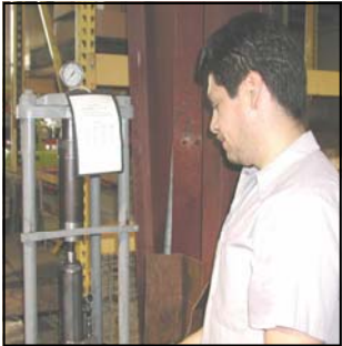
In this final phase of production each bottle jack and long ram jack is pressure tested by qualified personnel.
